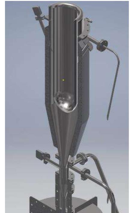
*Beam-down system and solar calciner designed in SOCRATCES*
