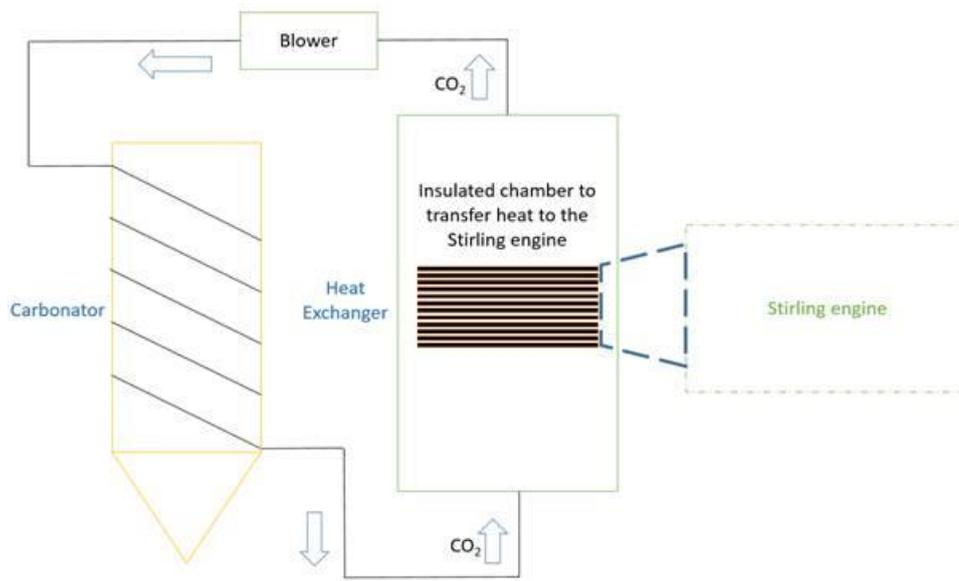
**Figure 17: Pictorial representation of the scheme of integration between the carbonator and the power block**
