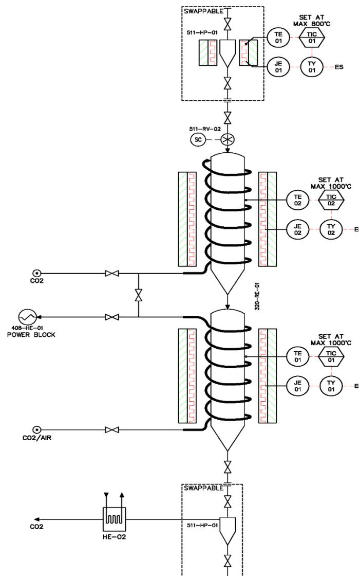
**Figure 11. Indirect integration scheme – SOCRATCES prototype. Preliminary design scheme of the carbonator reactor (figure developed by CERTH)**
