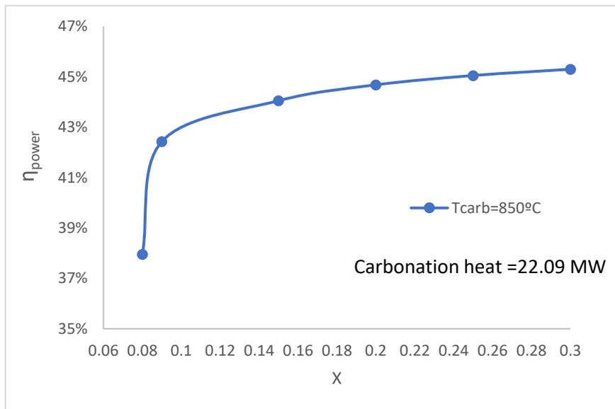
**Figure 9. Variation of carbonator side efficiency as a function of CaO conversion (X)**
