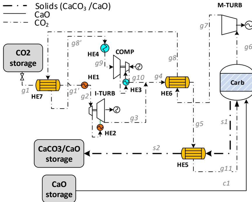
Figure 3: High-temperature solids storage. Direct integration. (HT-D) scheme
