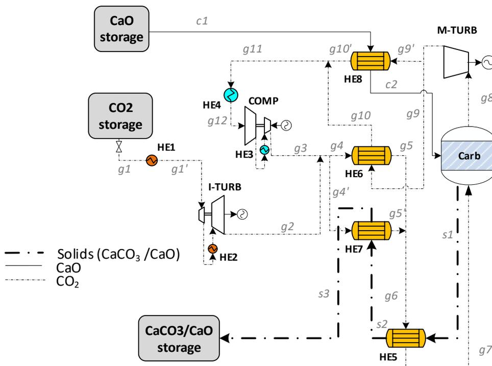
**Figure 8. Low-temperature solids storage. Direct integration (HT-I). Adapted from [5].**
