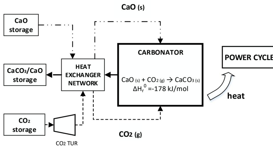
**Figure 1. Conceptual CSP-CaL process integration scheme for the carbonation side**
