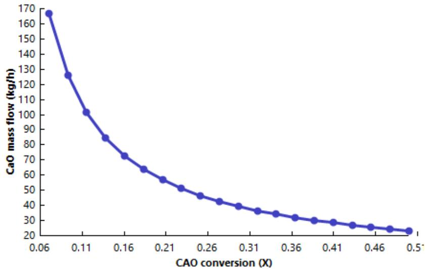
**Figure 13. CaO mass flow to the carbonator to achieve 10 kWt released in the carbonation as a function of CaO conversion in the carbonator**
