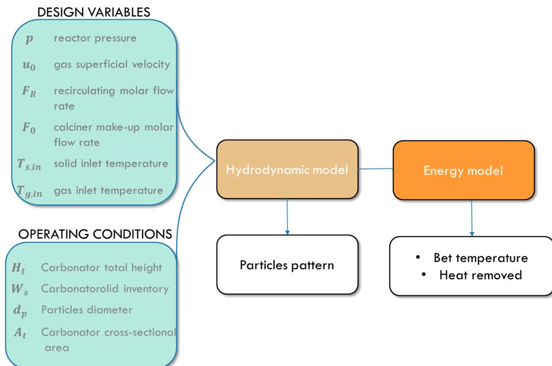
Figure 15. Structure of the carbonator model
