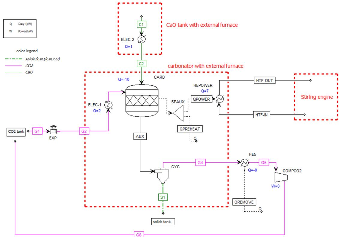
**Figure 12. Carbonator-power cycle for SOCRATCES prototype. Aspen simulation flowsheet.**
